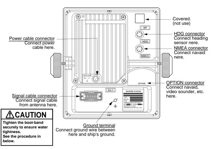
Figure 5-12 Display unit, rear view
